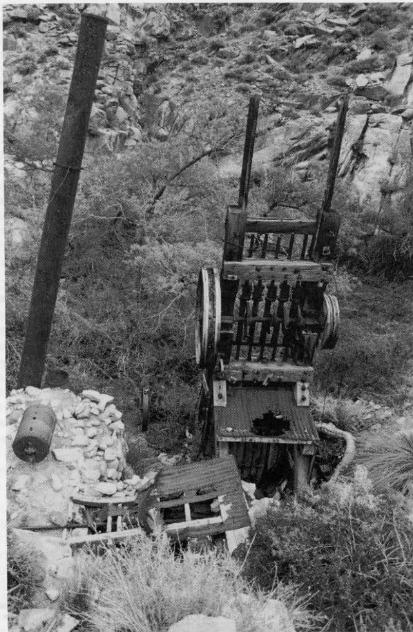
Five-stamp mill. The rock pile covers a boiler which fed a steam engine to power the mill.
